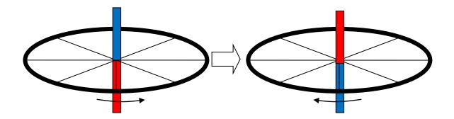
The wheel is turned upside down in 2.0 s. The magnitude of the angular momentum of the wheel stays the same. Calculate the average torque that was exerted on the wheel.
